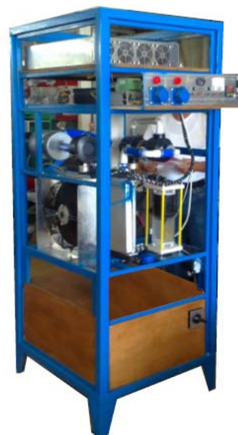
On the above photo is the fully automated 5kW powered PEM Fuel Cell System that uses as fuel Reformate Hydrogen from the Ethanol Reformer.
