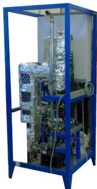
On the above photo is the Ethanol Reformer that has been used on the wine distillery. From this Ethanol Reformer, hydrogen is extracted and feeds the PEM Fuel Cell System
