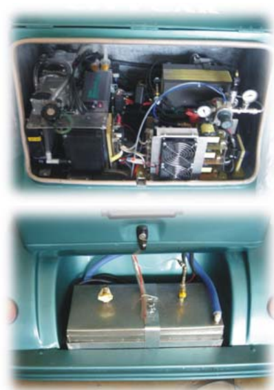
Tropical's Hybrid-Fuel Cell CityCar. Fuel cells engine (on the box) and hydrogen water cooled metal hydride tank (at the bottom)
